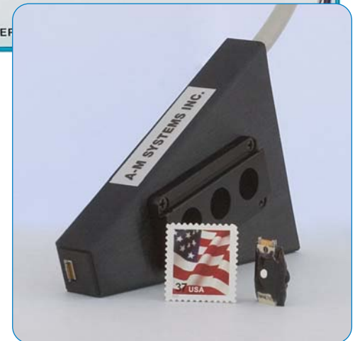
Stimulate & Record Headstage (left rear) Record-Only Headstage (right front)
